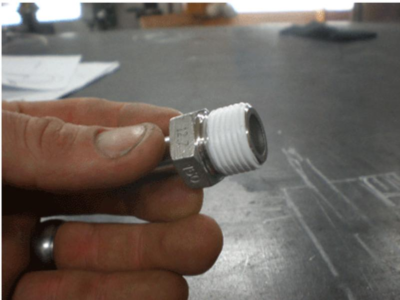
The fitting taped ready to be screwed into it's female counterpart.
